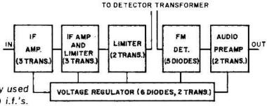
Fig. 2. This RCA IC is presently used in both FM and TV (sound) i.f.'s. It now becomes possible to have a complete i.f. in a TO-5 can (except for tuned circuits). In the not-too-distant future, it is likely that the entire FM set (and the bulk of the TV set), will be found in one tiny can!
