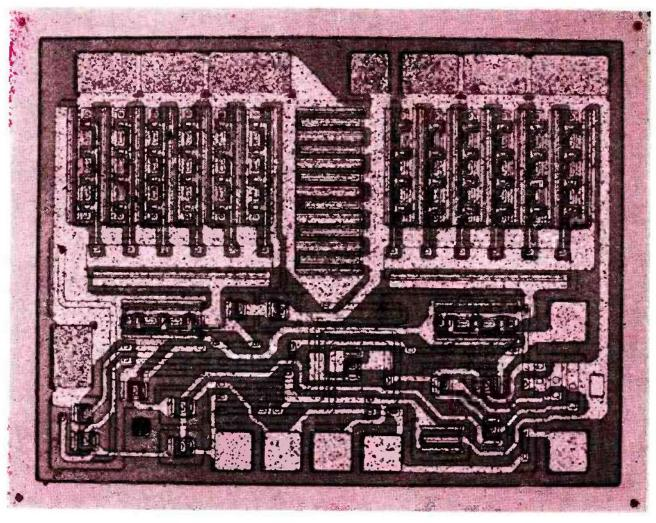
Because this 29-transistor, 14-diode receiver was designed and built in 1964, it does not use integrated circuits. It weighs only  $12\frac{1}{2}$  ounces and the entire unit occupies just 13 cubic inches of space.
